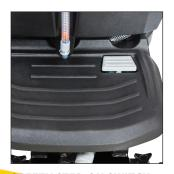
**SAFETY STEP-ON SWITCH** will only allow the unit to move when the operator is in the operating position.
